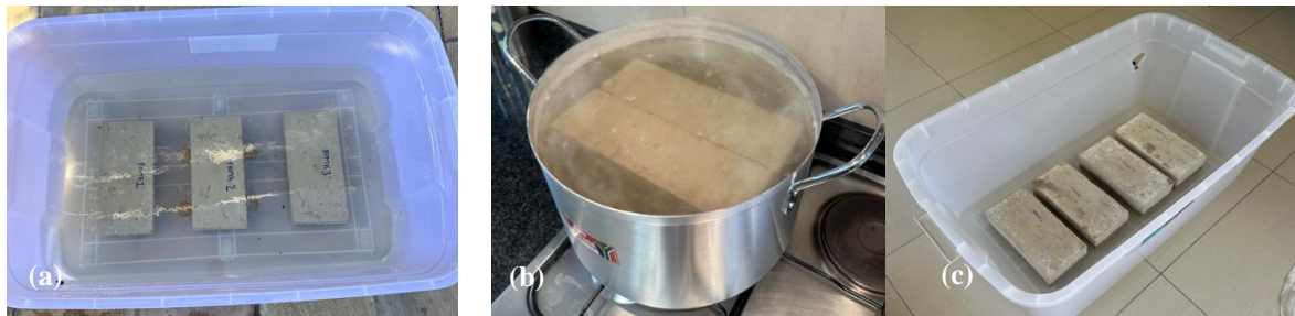
Fig. 3: Water absorption tests. (a) cold water, (b) boiled water, (c) IRA
