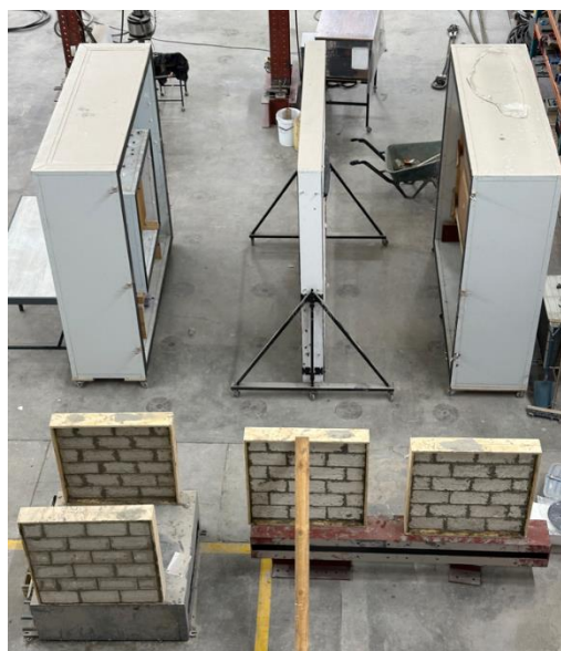
Fig. 4: Guarded Hotbox set-up
