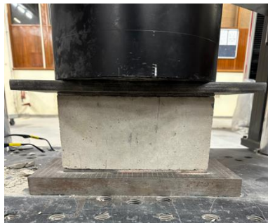
Fig. 2: Compressive strength test
